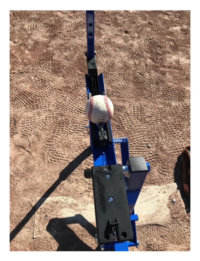
MICRO ADJUSTMENT SCREW: Screw clockwise to lower pitch, Screw counterclockwise to raise pitch. (This should be the only adjustment needed each game)
