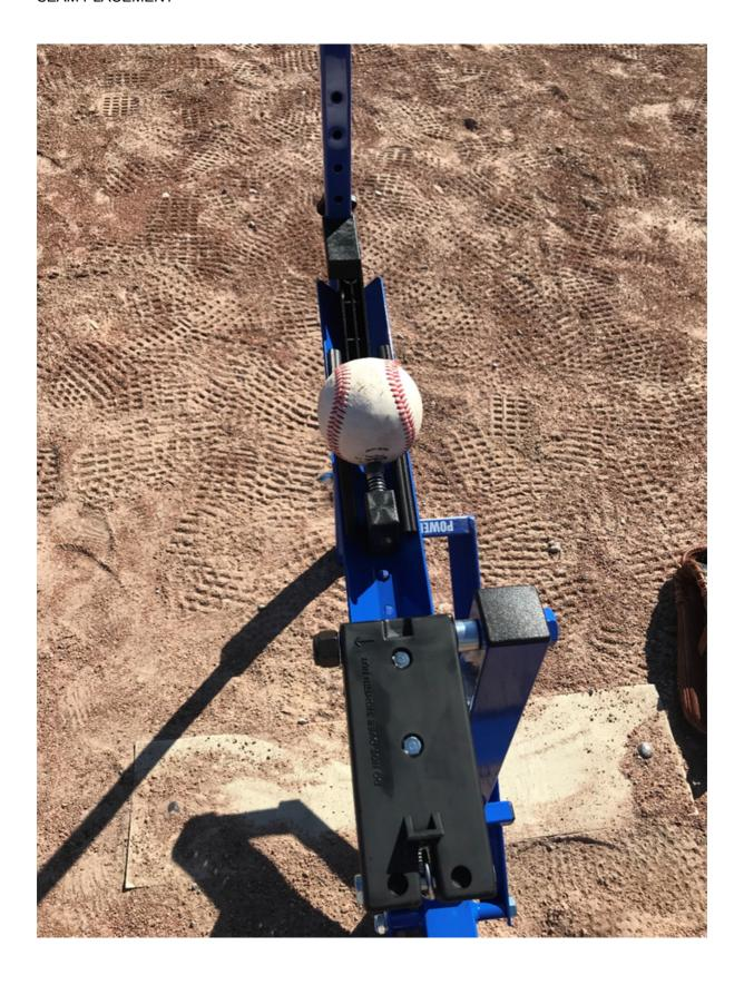
MICRO ADJUSTMENT SCREW: Screw clockwise to lower pitch, Screw counterclockwise to raise pitch. (This should be the only adjustment needed each game)
